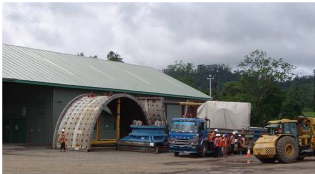
Figure 3: SAG mill sections and refurbishment workshop
